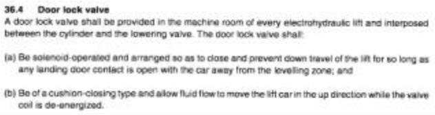
Interestingly this is only in these Australasian passenger lift standards and not reflected in either EN81 or the American standard A17 for electro-hydraulic lifts. Maybe this is because of the slower speeds of hydraulic lifts or that it has never been experienced as a problem.
