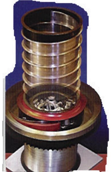
For 152mm dia. a maximum lift of 3.6 m is possible, whereas with the big mother 457mm dia. A height of 12.2 m is attainable. Speeds range from 0.1m/sec to 0.2m/sec and static loads of up to twice the lifting loads are possible.
