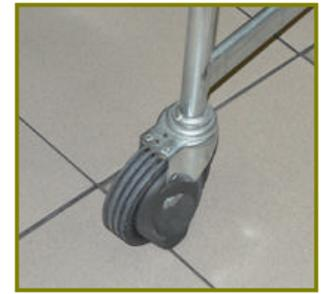
2. Only rear wheels should have discs fitted to align the trolley's locked wheels with the pallets. Discs on the front rotating wheels if set before the rear ones, mean the rear of the trolley cannot set without the need to be moved laterally to align them with the front wheels to provide the preferred exiting push from the rear.
