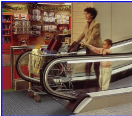
shopping trolley up the incline. She became concerned when the tyre of one wheel began to peel off into the mechanism. Because of the friction against the balustrade the tyre eventually peeled off, and the resulting now uncontrollable trolley eventually turned and jammed between both sides of the balustrades.
